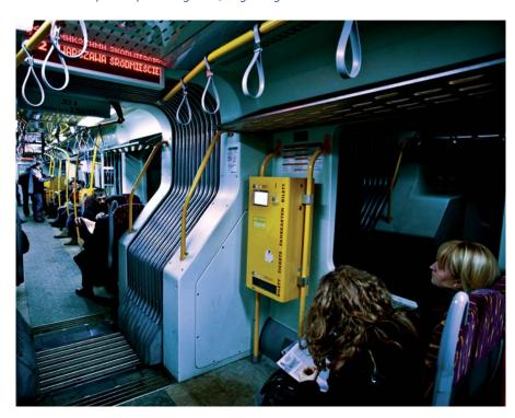
Electronic displays inside the vehicle have become a standard piece of equipment in the new public transport buses and trams. The dynamic display located by the middle door shows the route; the part already travelled shows grey. Outside displays give even more information (about the terminus, the bus going to the depot, or changes in the route).
