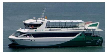
The new catamaran ferryboat has a length of 25,8m and welcomes 150 passengers. The main deck is fully adapted to passengers in wheel chair.
