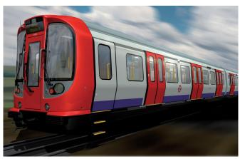
The 'S-Stock' trains, which will serve around 40 per cent of the Tube network on the sub-surface lines, will have air conditioning, walk-through carriages with CCTV coverage in each one, plus improved accessibility. They are being delivered as part of TfL's Investment Programme.
