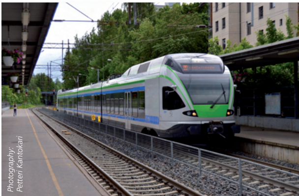
The Helsinki Sm5 FLIRT is 75m long EMU train unit with 4 sections and 6 low-floor entrances. The passenger capacity is 260 seated, 380 total. The top speed is 160 km/h, and the train has a high rate of recovery both for driving and heating energy, making it suitable for the Finnish conditions.
