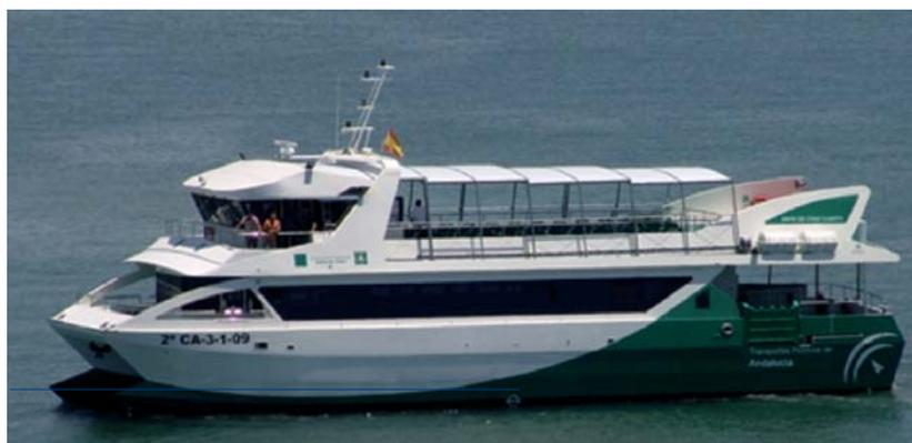
The new catamaran ferryboat has a length of 25,8m and welcomes 150 passengers. The main deck is fully adapted to passengers in wheel chair.
