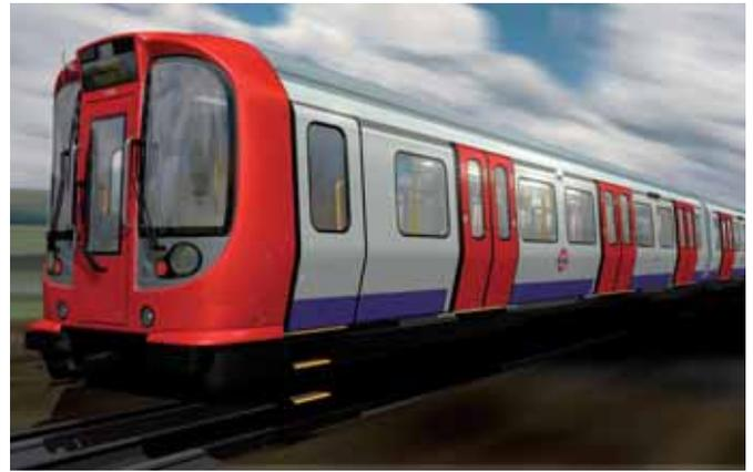
The 'S-Stock' trains, which will serve around 40 per cent of the Tube network on the sub-surface lines, will have air conditioning, walk-through carriages with CCTV coverage in each one, plus improved accessibility. They are being delivered as part of TfL's Investment Programme.
