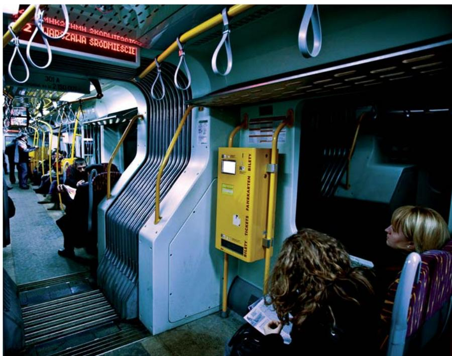
Electronic displays inside the vehicle have become a standard piece of equipment in the new public transport buses and trams. The dynamic display located by the middle door shows the route; the part already travelled shows grey. Outside displays give even more information (about the terminus, the bus going to the depot, or changes in the route).
