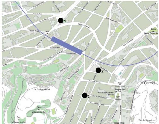
The recently inaugurated segment of L5 includes the station at El Coll | La Teixonera, close to Parc Güell. It was constructed on a particularly difficult site. As a result, this station is the deepest in the whole network, with a maximum depth of 104 m below street level.
